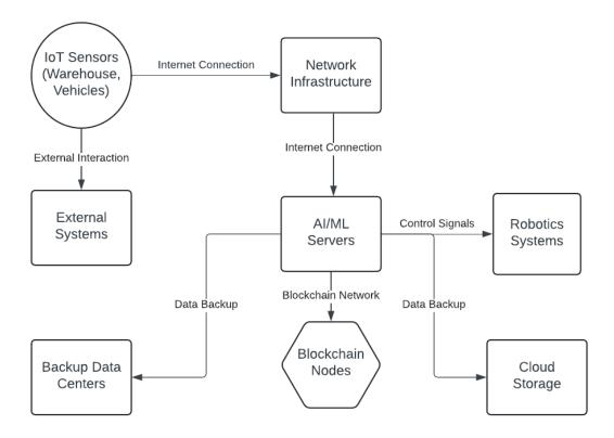
*Note. The network architecture and hardware configuration of FedEx's upgraded system are shown in Figure 5.*
